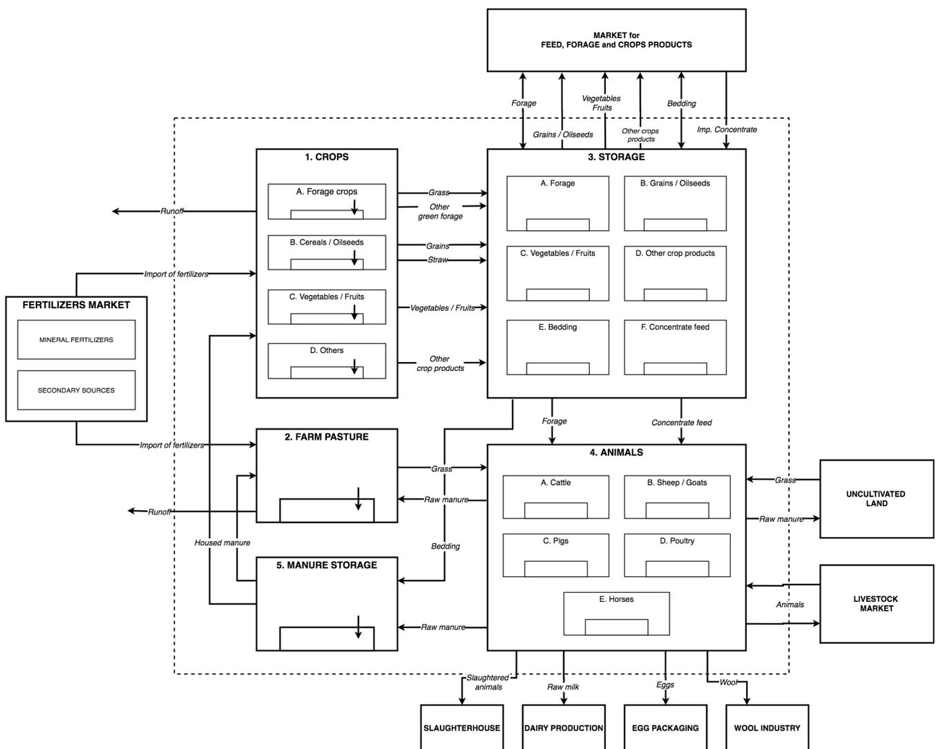
**Figure 3: Disaggregated system definition.** The *Crops*, *Storage* and *Animals* processes are divided in subcategories. This representation of the system definition also features external processes, like *Uncultivated land* or *Slaughterhouse*.
